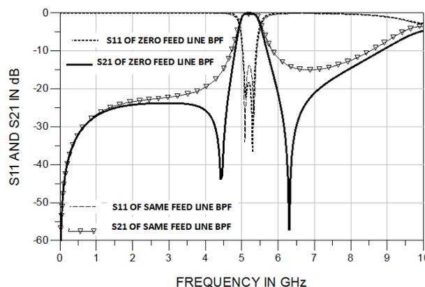
**Fig.3** Comparison of simulated result of BPF using two feed line structures
