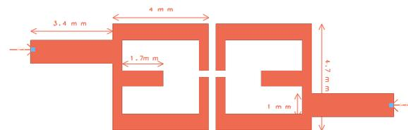
**Fig.1** Open loop resonator using zero-phase feed line Filter Structure
