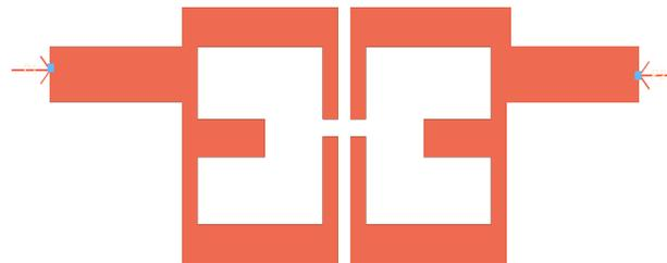
**Fig.2** Open loop resonator using same-phase feed line Filter Structure
